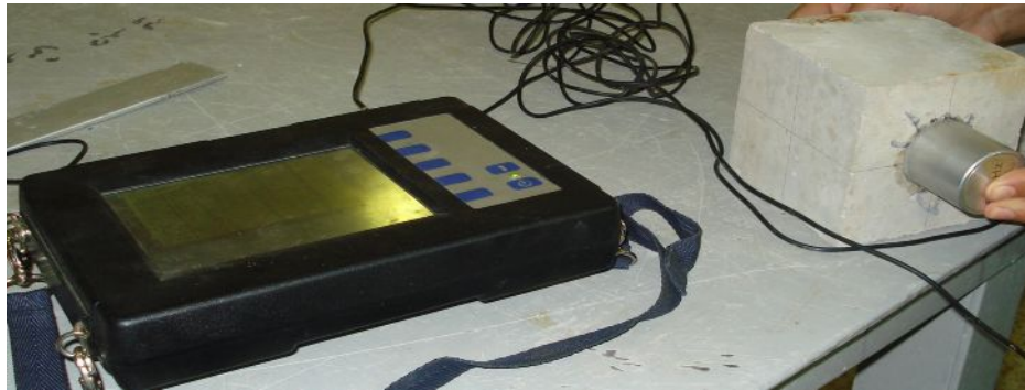
Fig.(11): The arrangement used for the ultrasonic pulse velocity measurement.
